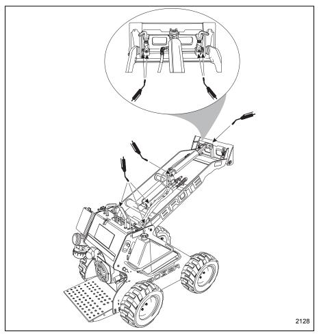
Figure 4-9 Lubrication Points
